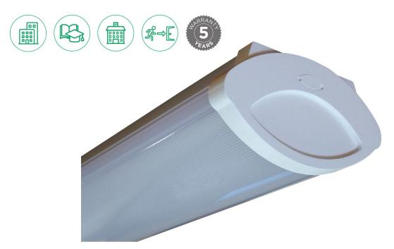
An IP20 luminaire with dry powder coated steel base, opal polycarbonate internal ridged extruded diffuser and polycarbonate end caps, with surface and suspension mounting capabilities. Digital dimming and integral emergency versions available.
