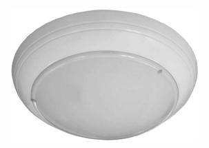
A range of surface mounted decorative anti-ligature luminaires. Constructed from a spun aluminium circular base, with opal polycarbonate diffuser. Suitable for use in corridors, reception areas, hospitals, schools, secure bedrooms and other internal areas.
