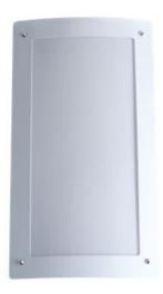
A distinctive and attractive slimline luminaire with slotted side panels which give a subtle horizontal back light. Fabricated from white dry powder coated mild steel base/ diffuser frame and opal polycarbonate diffuser secured by decorative chrome bolts. Suitable for hotels, offices, corridors and stairwells.
