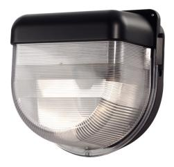
Exterior amenity wall light. Black polycarbonate visor, clear prismatic polycarbonate hinged diffuser, black die-cast aluminium base.
